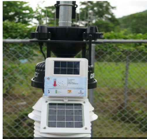
An automatic weather station installed at Mona Dam. Photo: Planning institute of Jamaica, 2018
