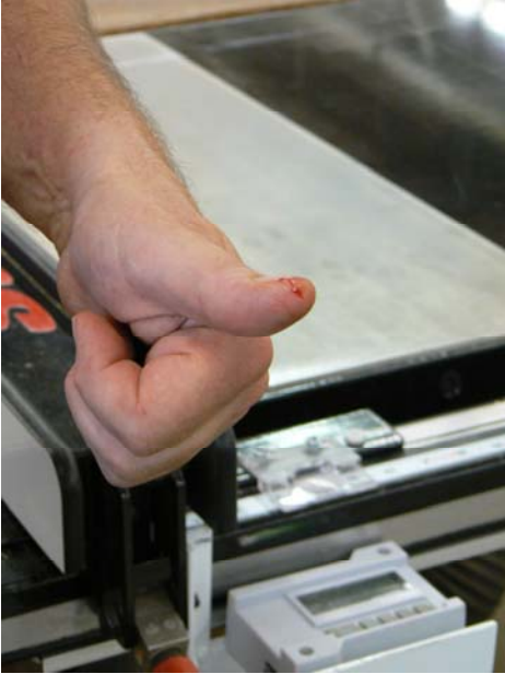
Robert right after his thumb came in contact with the blade while using a SawStop Industrial Grade cabinet saw in July 2006.
