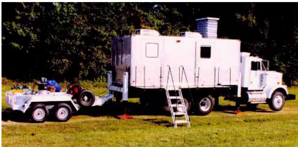
Figure 1. SCAPS Truck Photo with Trailer for Grouting
