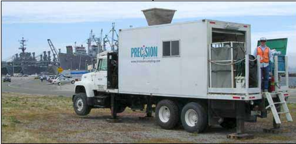
Figure 10. Photo of Precision Sampling Truck for Cone Penetrometer Technology
