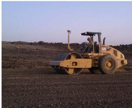
Shown is NorthGate equipment utilizing the intelligent compaction software, with the receiver at the top.
