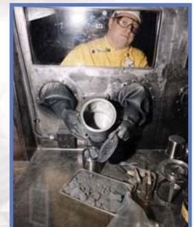
More than 1,457 contaminated glove boxes (stainless steel enclosures where workers handled nuclear materials) were cleaned and removed.
