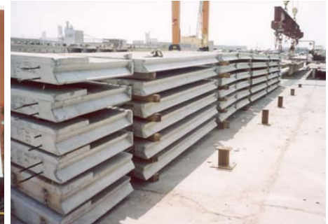
Fig. 9. Storage of NUDECK Panels in the Precast Yard
