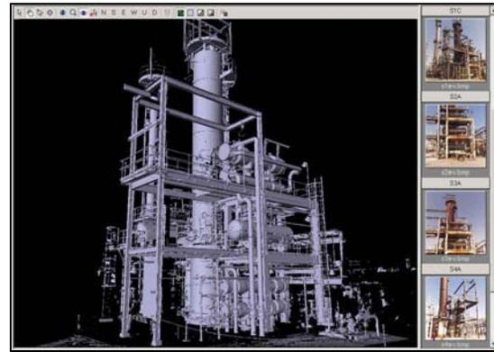
Figure 3 - Optimized 3D Surface Model
