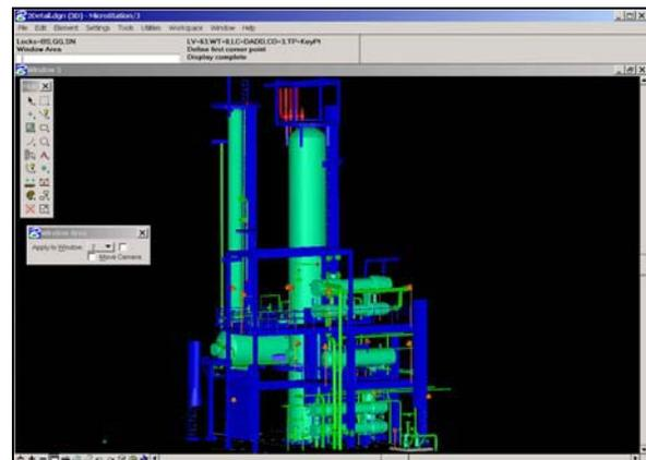
Figure 5 - Complete CAD Model from laser scanning (No longer needed)
