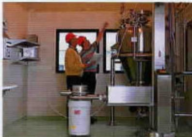
Process and utility equipment is installed in Sweden. A pre-IQ and test-run is performed to secure the quality.
