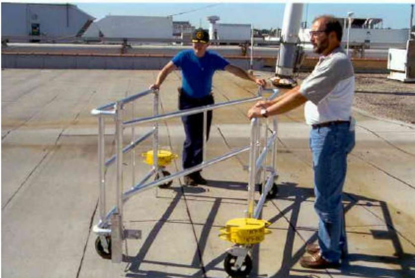
Mobile Parapet Barrier being opened.
