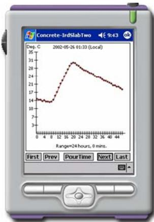
A sample of the temperature log as displayed on the handheld PC.
