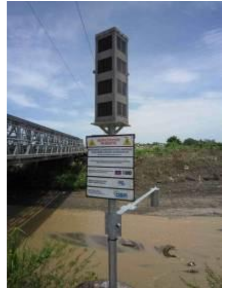
Limnimeter on a bridge in Port-au-Prince
